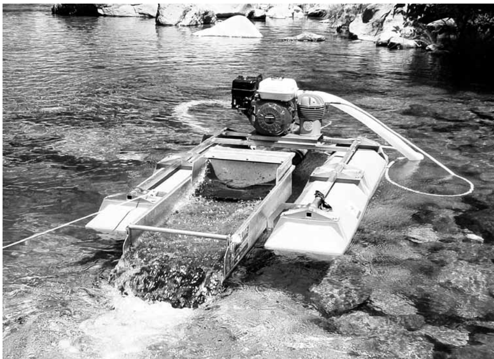
Floating suction dredge. Photo courtesy of Western Mining Alliance.
