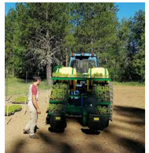
Luke Doyle plants new hemp starts using a water wheel planter at Murphy Hemp Company. Photo: Kit Doyle.
