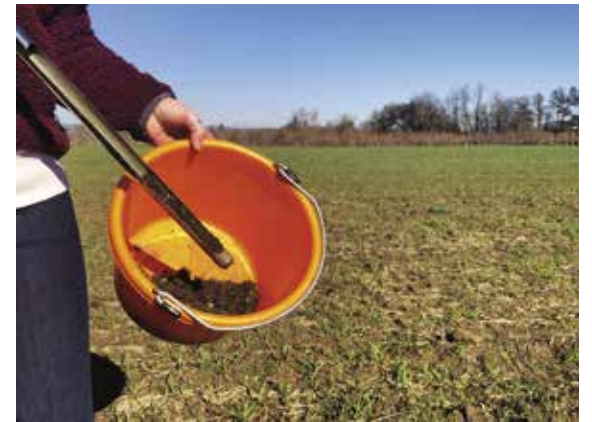
Combine 15 to 20 soil cores from each area of your property to get a representative sample for analysis.
